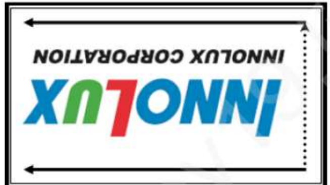
Fig. 2 Reverse scan (PCBA on the bottom side) ( pin 17, REV_SCAN = High )
